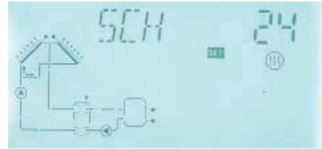
Other temperature difference between T6 and T2 ( $\Delta T1$ ), it can heat tank through P2.
