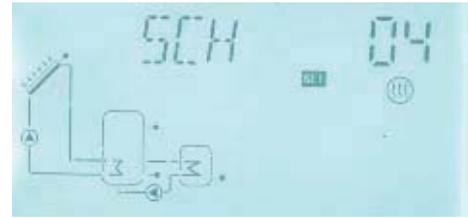
Other temperature difference between T3,T4 ( $\Delta T2$ ) controls pump 2 to transfer heat from tank 1 to tank 2.
