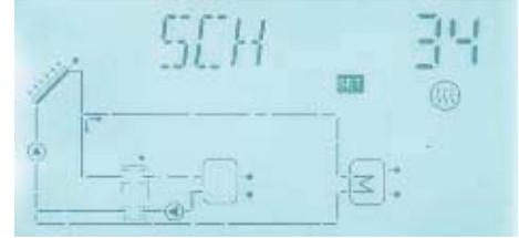
Other temperature difference between T6 and T2 ( $\Delta T1$ ) controls P2 to heat tank 1.
