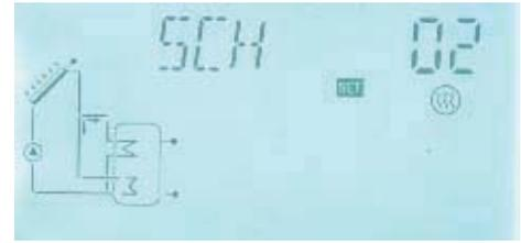
Priority logic controls the top zone of tank is prior to heated, this is default factory set, impossible to be changed.
