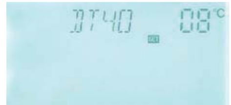
▶ Press **+** **-** button to adjust switch-on temperature difference, adjustable range (OFF+2 °C) ~20 °C, factory set: 8 °C
