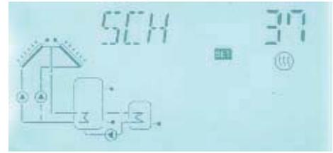
Other temperature difference between T3 and T4 ( $\Delta T2$ ) controls R1 to transfer heat from tank 1 to tank 2
