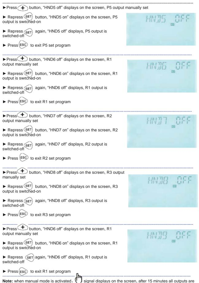
**Note:** when manual mode is activated, **V J** signal displays on the screen, after 15 minutes all outputs are switched-off, controller exits manual mode automatically.
